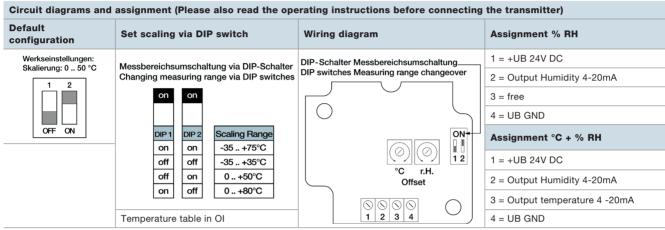
The humidity path must be connected for the current version! Please refer to the operating instructions for the correct connection.
