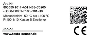
Label for cable probes (attached to the cable as a flag)
