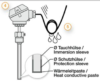
Please lay the cable so that no water can penetrate the probe and with a spare loop (4). This allows you to extend the probe without disconnecting the electrical connection.
