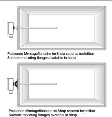
Mounting by means of mounting flange: Please make sure that the Ø of the mounting flange matches the Ø of the protection sleeve. Suitable flanges can be found at testo-sensor.store.
