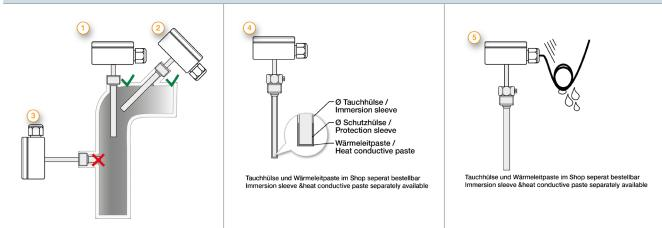
Measurement errors can occur due to heat dissipation to the environment. To keep these as small as possible, we recommend immersing the protection sleeve of your temperature probe as deeply as possible in the medium to be measured during installation. The optimum installation depth should be 10-15 times the Ø of the protection sleeve. Please make sure that you have sufficient space so that you can remove the probe again if necessary.
