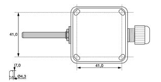
Thanks to the four slotted holes, the housing can be easily mounted on the wall. The openings for the screws are located outside the protective space for the electronics, so no sealing is required. With the cable compression glands, sealing to the probe or data cable is guaranteed even for different diameters.
