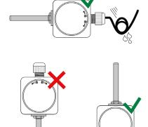
Mount your outdoor probe with sufficient distance to vents, windows or doors and preferably on the north wall, alternatively on west or east wall of the building. Avoid direct sunlight and rain. Use Sun Protection if necessary. Please lay the cables downwards so that rainwater can drip off in a defined way. Please consider the permissible ambient conditions during installation.
